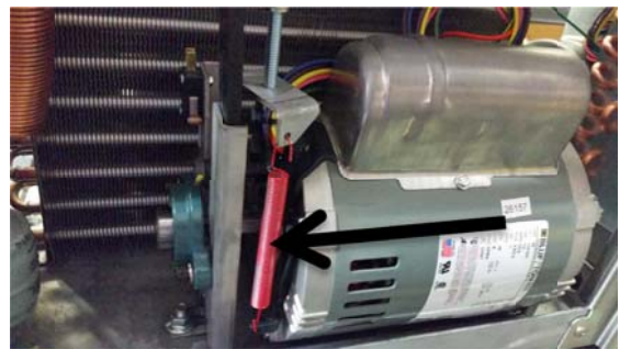
Replace Spring (if equipped) with same color Spring
