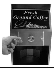
8. Set brew basket stop for size brew baskets being used. There are three basic sizes for the brew baskets: 7-½ inches, 7 inches, and 6 inches. This dispenser is set for a 7 inch brew basket. If you're using a different size of brew basket, remove the two screws holding the brew basket stop and move stop to the location corresponding to your brew basket size.
