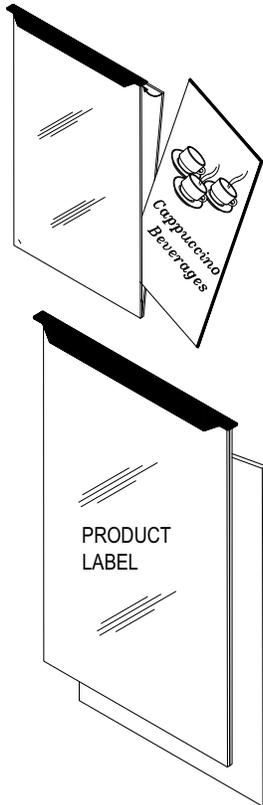
1. Lift up the two end tabs on top of door with a pointed object or flat head screwdriver.
