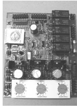
61800 PIC 2/3/5/6 Controller NOTE: PIC5 & 6 use 2 controllers
